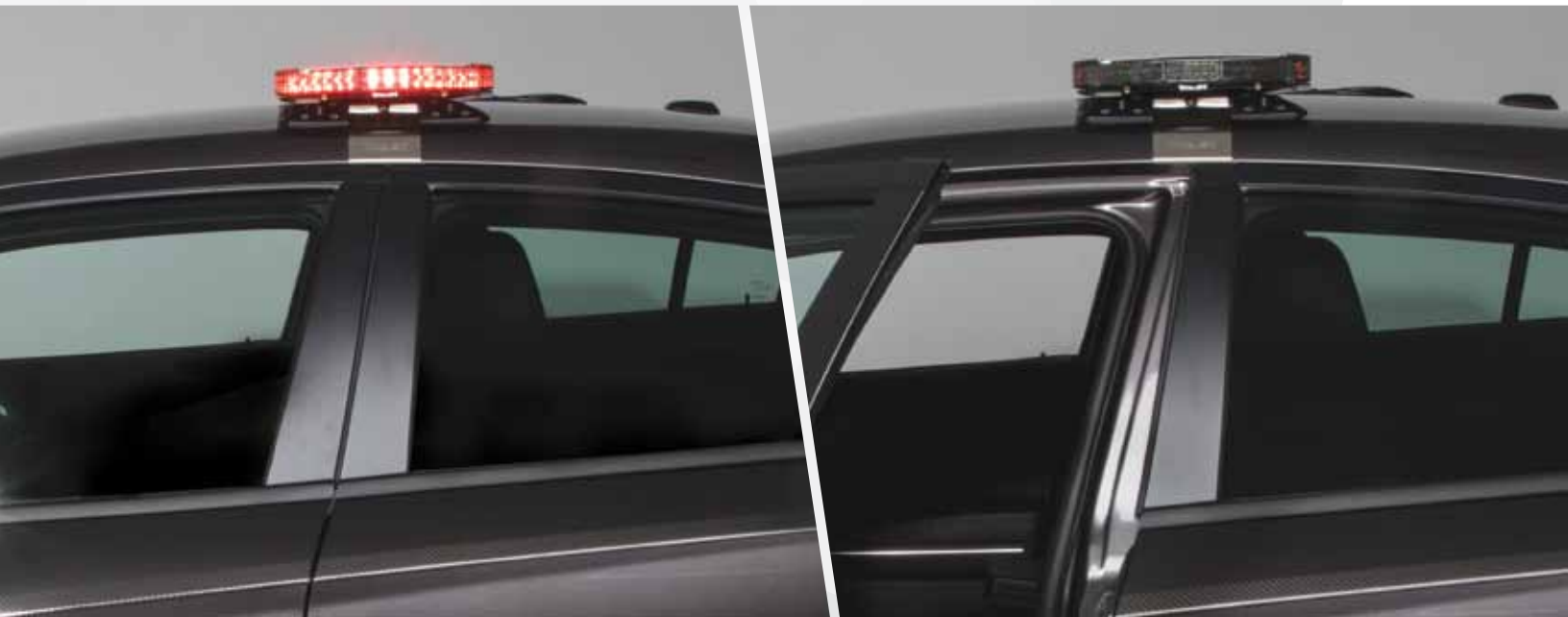
Turn off end warning/alley lights when door opens
